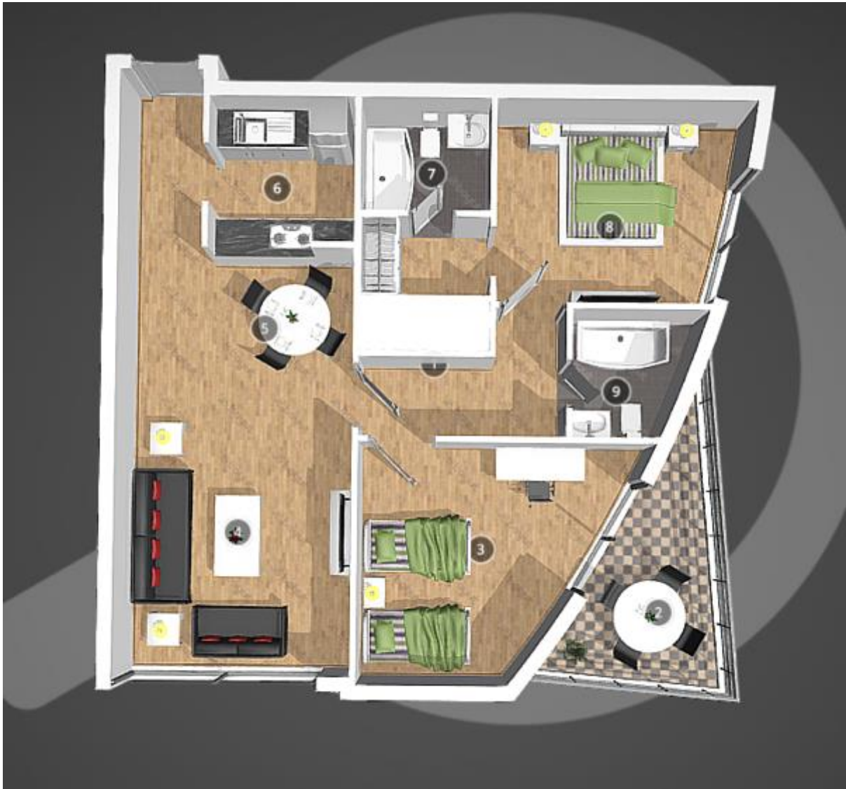
Figure 22: The plan showing the layout of the flats on the 15 th floor, where the outer wall on one side follows the curved profile of the fins. The fully-exposed triangular balcony is at the top of the glazed corner section. Image: www.bayut.com
